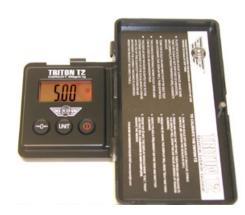
The scale should be on the desk with the cover removed and used as a tray resting on the measurement pad. The protective cover of the Triton is designed to also be used as a tray. The cover can only be removed when the scale is fully open. Fully open the scale to unlock the cover and slide towards the left of the scale.
